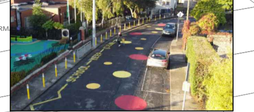
PAINTED ROUNDELS IN SCHOOL ZONE AS PER NTA SAFE ROUTES TO SCHOOL DESIGN GUIDE
