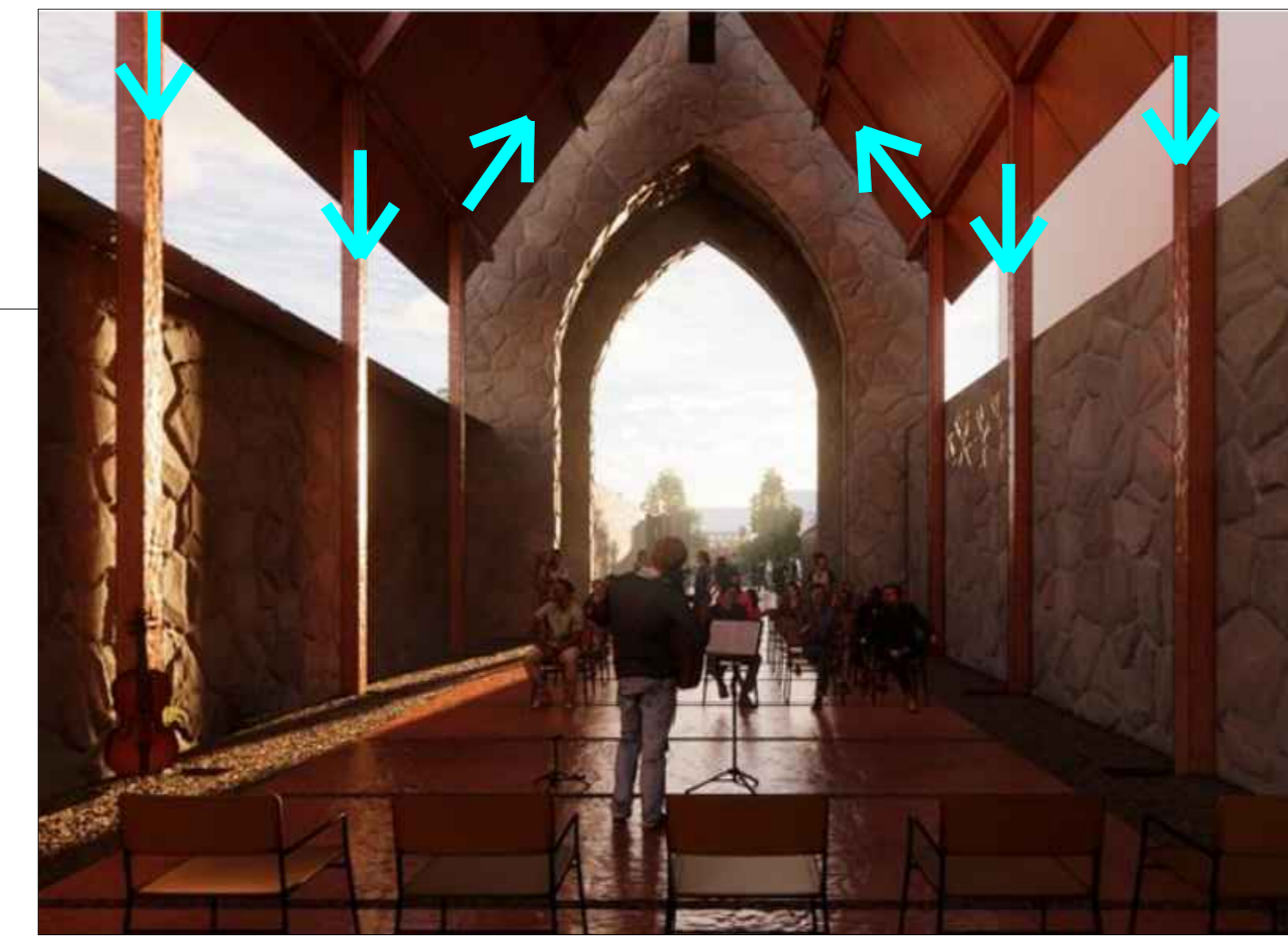
FEATURE LIGHTING - SCHREDER VALINTA LED SPOT LIGHT MOUNTED ON ABBEY LIGHT ROOF SUPPORT STRUCTURE TO HIGHLIGHT THE EAVES AND INTERNAL SPACE. EAVES TO BE ILLUMINATED BY PHOTOCELL. DOWNWARD SPOTS TO HAVE LIGHTING CONTROL SWITCH FOR WHEN SPACE IS USED FOR EVENTS.
