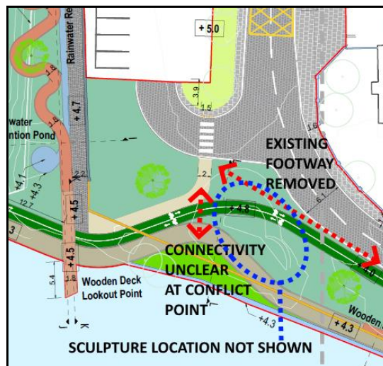
Figure 5: Existing Sculpture, hedges and footway to be removed To construct cyclepath and Riverside Footway
