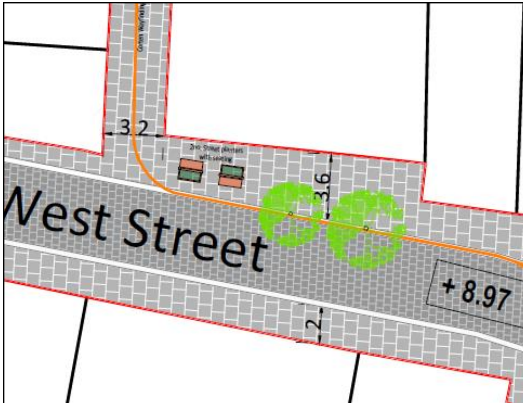
Figure 35: Planting located too close to carriageway edge
