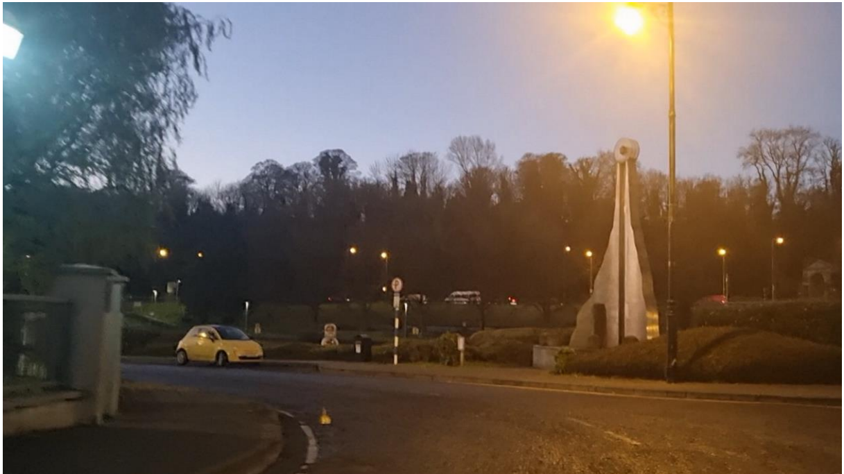
Figure 38: Nearside boundary Treatment reducing SSD 3 on Father Connolly Way
