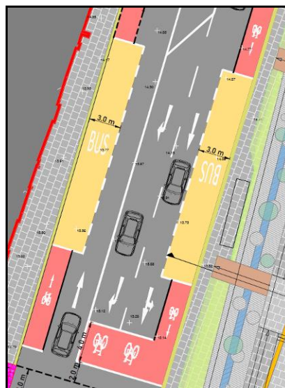
Figure 50: Narrow Lanes on George’s Street with No space for vehicles to pass stopped buses safely
