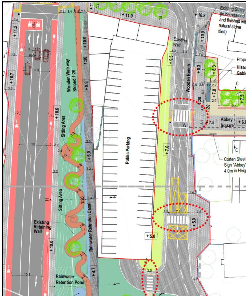
Figure 100: Inconsistent Crossing facilities and very narrow footways On Father Connolly Way
