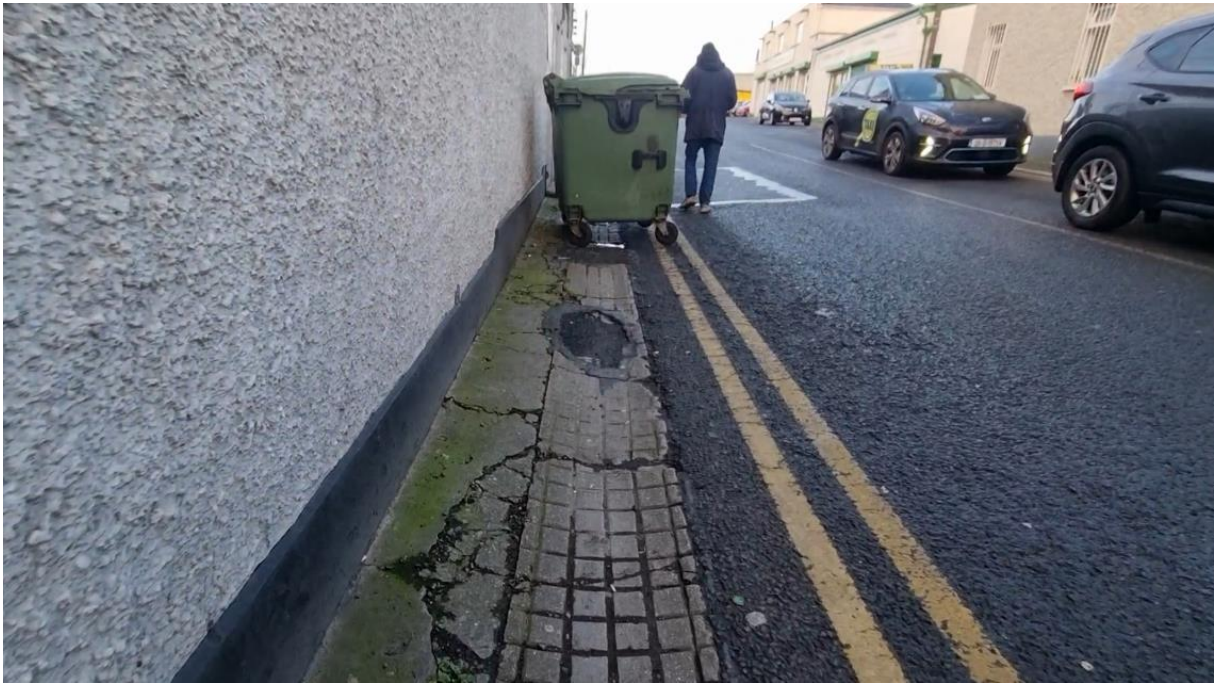
Figure 98: Pedestrians forced to walk in carriageway on Fair Green where additional obstructions arise
