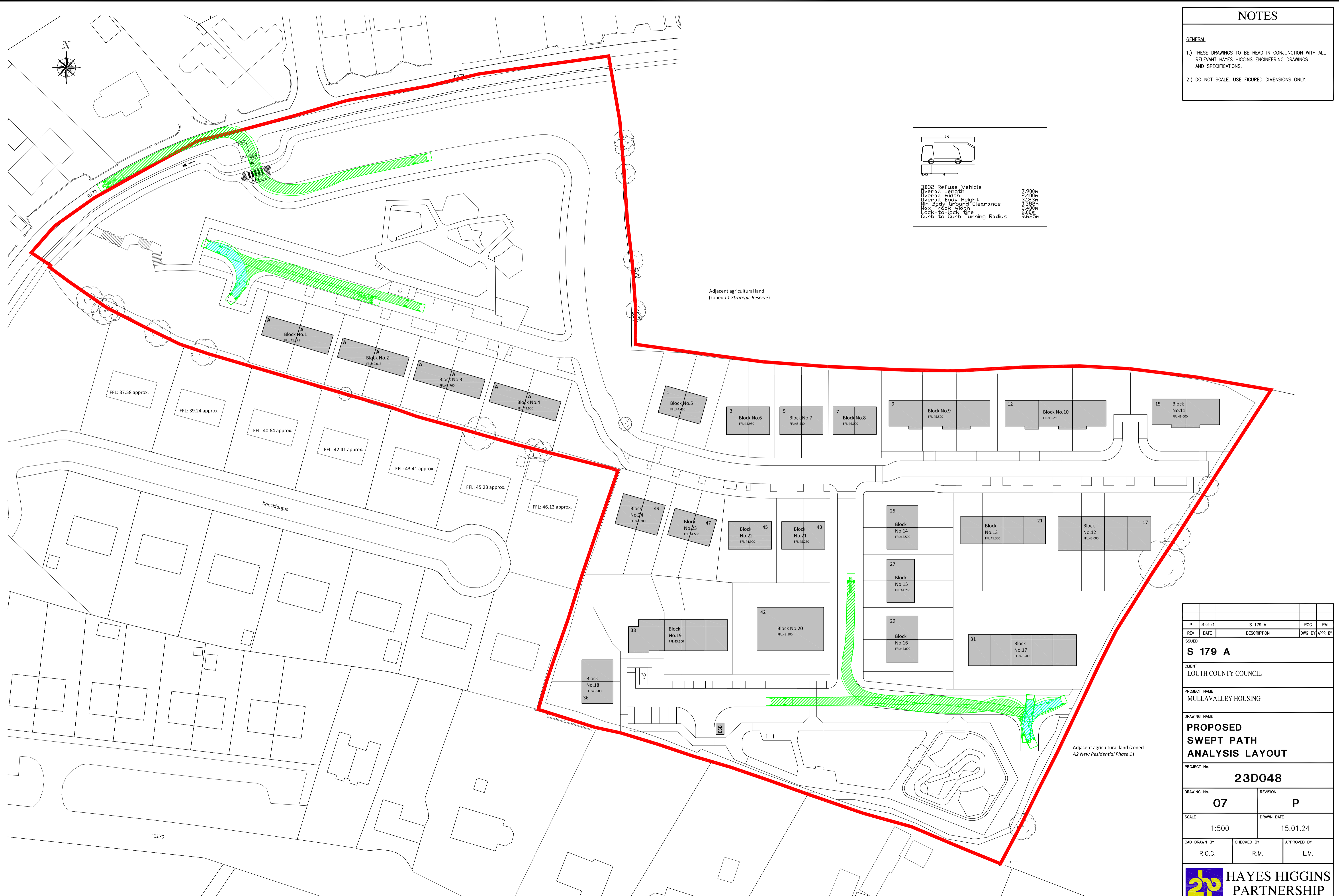
PROPOSED SWEEP PATH ANALYSIS LAYOUT SCALE 1:500
