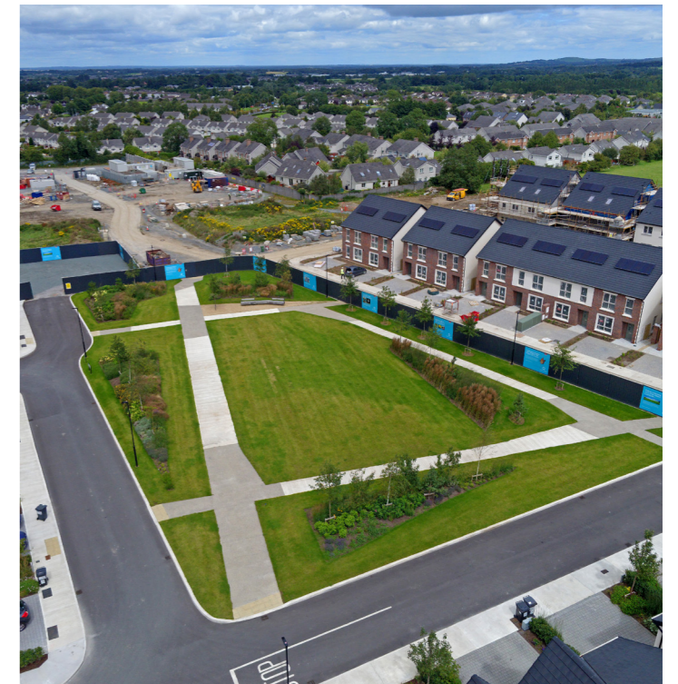
Material changes- used to highlight crossing points and to add variation in public realm materials
