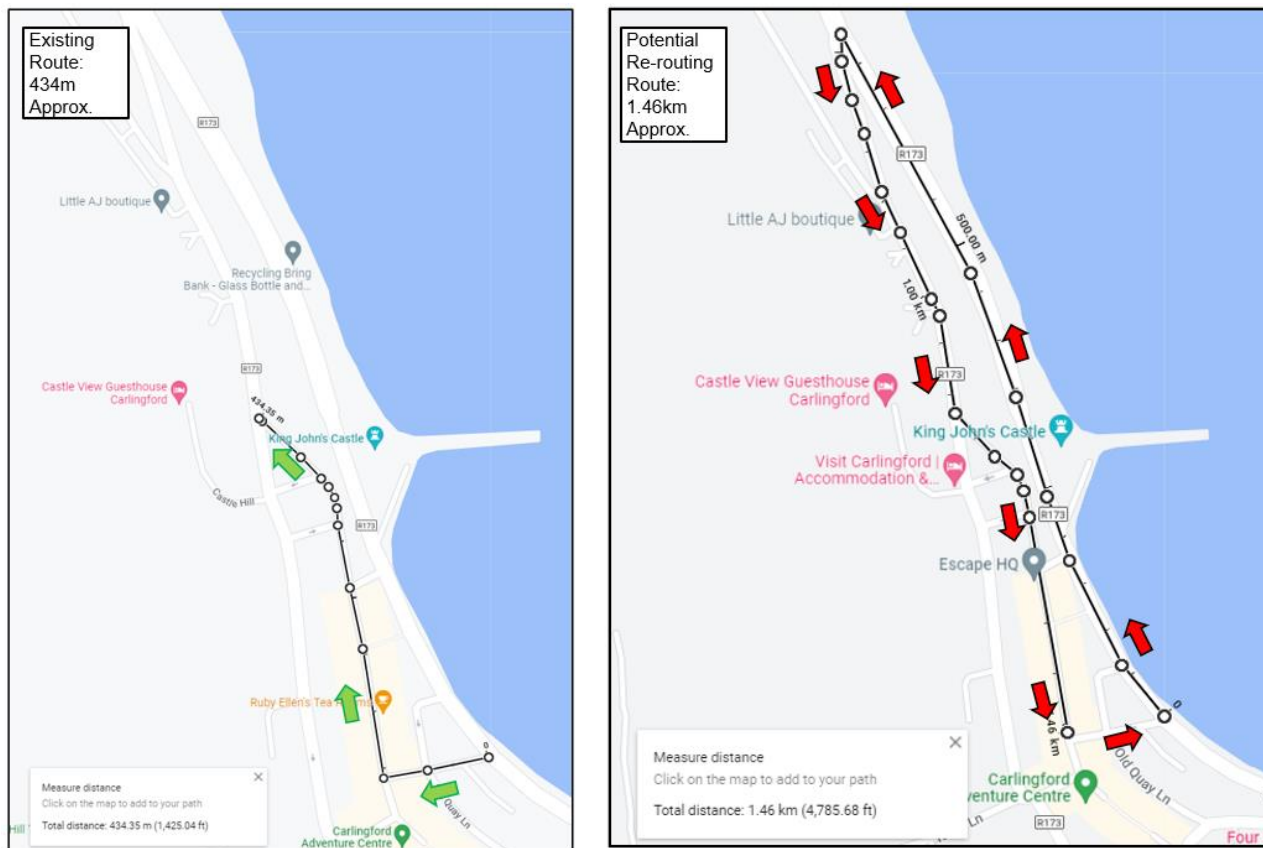
Figure 3-15 Considered Change to Traffic Flow Arrangement Analysis – Newry St.
